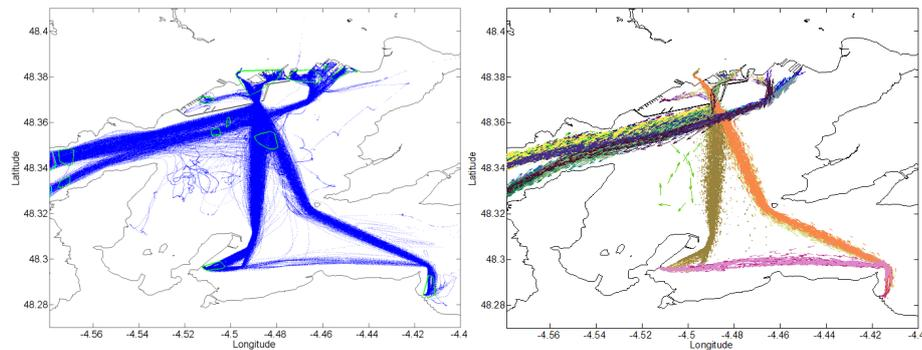
**Fig. 1.** Left: AIS positioning information (blue) and detected stationary (green), entry (cyan) and exit waypoints (magenta). Right: colour-coded oriented route objects.
